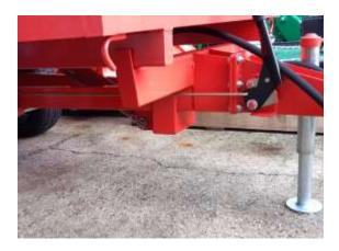
Align the tractor's rear drawbar to the pin hitch (2) on the trailer. Then raise or lower the trailer hitch using the stand (3). The handle can be used to wind the trailer up so the trailer and tractor hitching points are aligned. Then insert the tractor pin through the drawbar and trailer hitch to secure in place.
